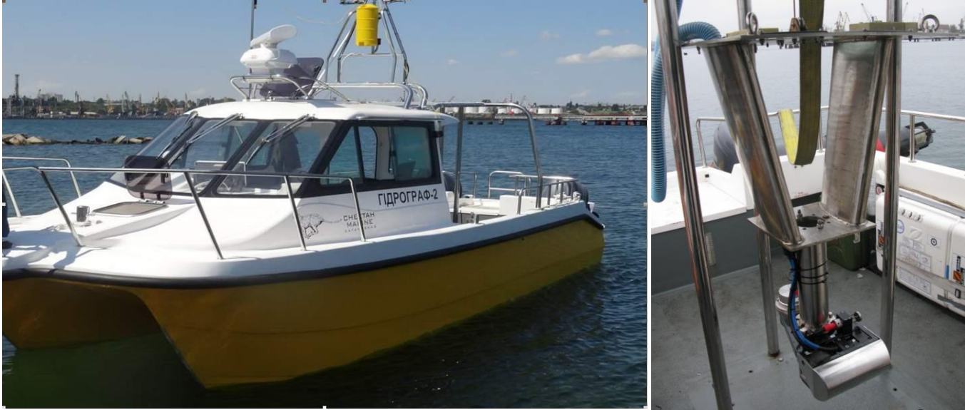
Small surveying catamaran (MGK-catamaran Hydrograph-2 ) with the onboard (ship borne) multibeam echosounder system
