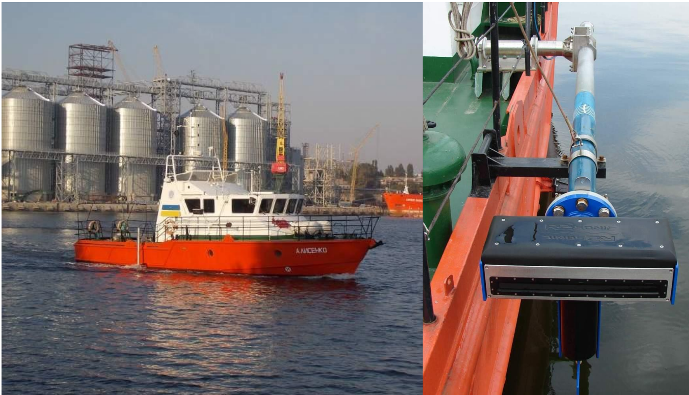
Big surveying vessel A.Lysenko with the multibeam system installed in 2016
